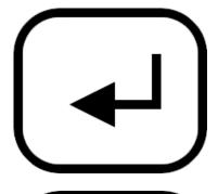
The ENTER button is used to select a blinking icon for changing. If a popup is open, the button is used to confirm the change. If no icon is blinking, the button will bring you back to page 1.
