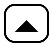
The UP button has three different functions. Navigating the page, increasing a value, and enabling a parameter.
