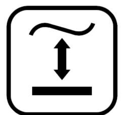
The MAIN button has two functions. Each time it is pressed, it switches the reel between three states, i.e., hauling, stop and pay-out. If the button is held for more than 5 seconds, the reel will enter a neutral state and release control of the drum, which can then be turned freely.
