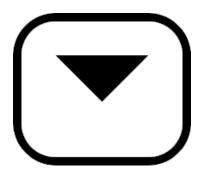
The DOWN button has three different functions. Navigating the page, decreasing a value, disabling parameters.
